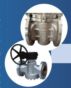
usefulness. The use of lubricant between the plug face and the seat eliminates most of these problems. The lubricant helps to control leakage around the plug, reduces wear between the valve contact surfaces, and slightly lifts the plug to reduce the operating torque required to operate the valve.
